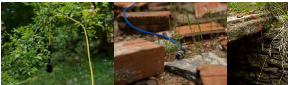
Figure 6. Wired microphones in several positions and ready to be plugged in Sanatorium, photos by Christos Schoinas (May, 2024)
