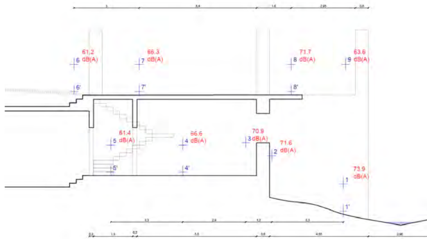
Figure 6. A comparison of all dB(a) at all selected positions, presenting a drop in every position
